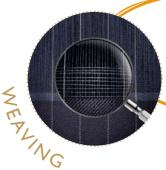
The transversal threads that make up the weave have to pass above and below the vertical threads of the warp, according to a precise schema. It is an incredibly precise and extraordinarily swift dance, turning thread into fabric in just a few short seconds.
